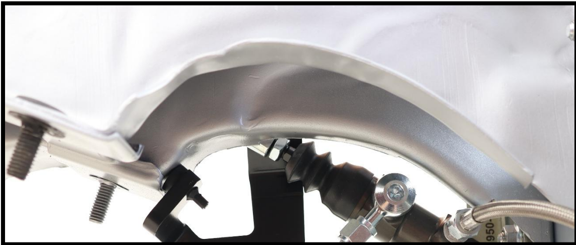
Pedal stop in pedal shown touching the pedal hanger and jamb nut loose on the master cylinder rod.
