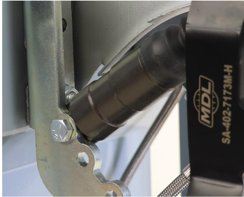
Master cylinder shown in UPPER mounting hole location.
